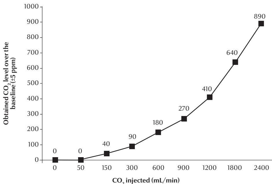
Figure 1 Flow concentration function for CO<sub>2</sub> 2% injection in the wind tunnel over the background level
