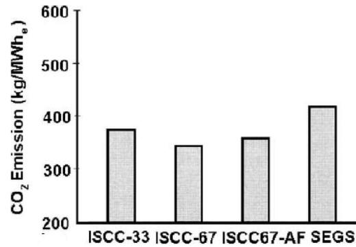
Figure 2. CO<sub>2</sub> emission per unit of produced energy for different cases [8].
